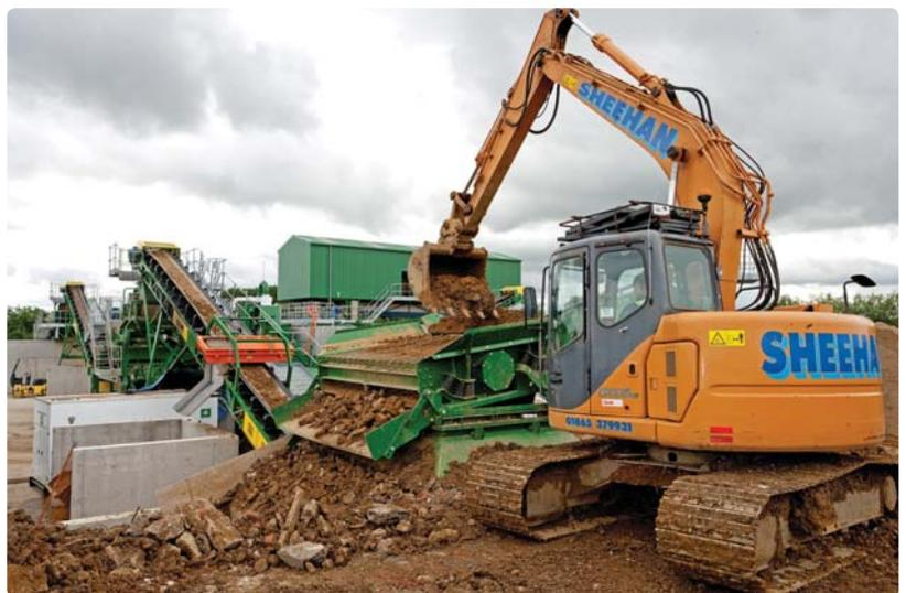
C&D waste being fed into the recycling plant.
